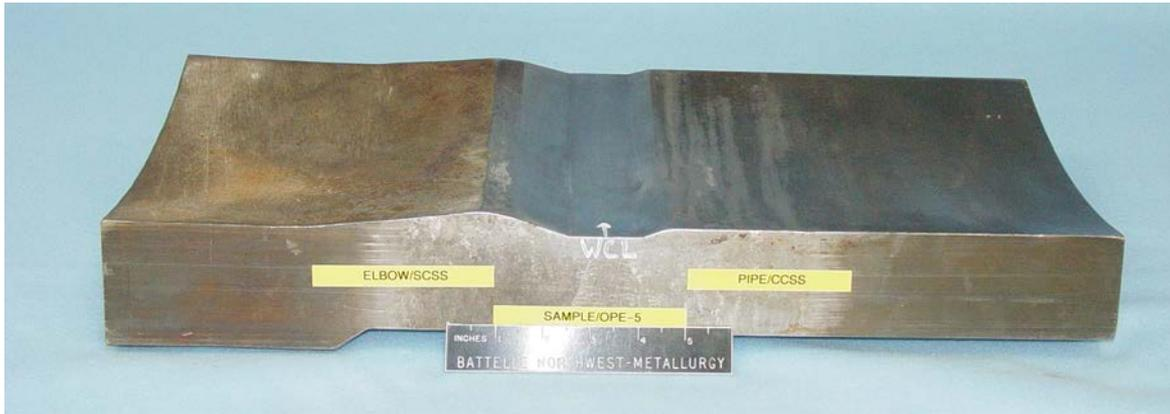
OPE-5, SCSS elbow 7.1 cm (2.8 in.) wall, CCSS pipe 5.8 cm (2.3 in.) wall
