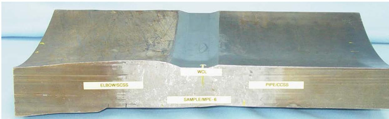
MPE-6, SCSS elbow 8.4 cm (3.3 in.) wall, CCSS pipe 6.6 cm (2.6 in.) wall
