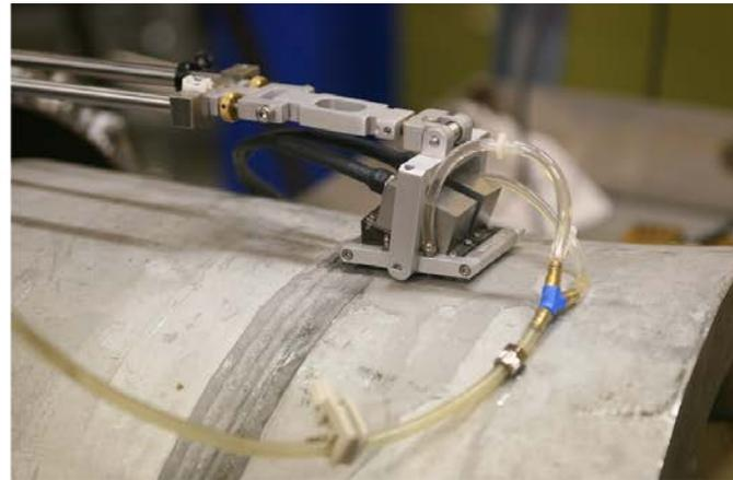
Scanner arm, probe and coupling configuration
