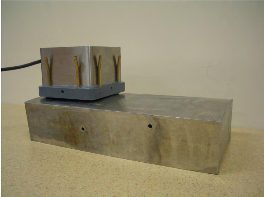
Dual 2D array probe, 0.5 MHz (Courtesy of PNNL)
